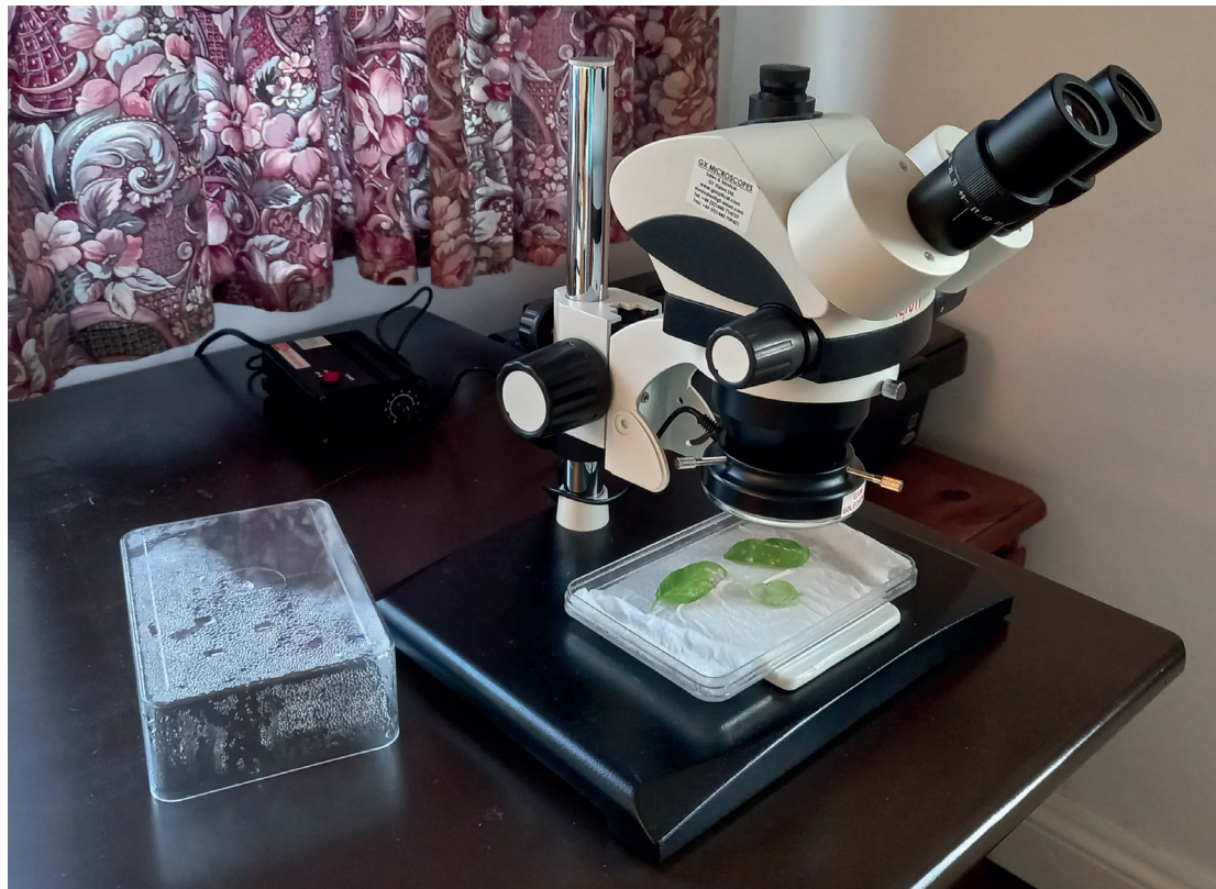
Fig. 7. Arrangement for viewing specimens on the lid of an incubation chamber.
