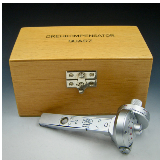
Fig. 41. A Carl Zeiss Ehringhaus compensator showing two graduated drums for precisely measuring the amount of tilt of the quartz plate, from which birefringence can be determined.
