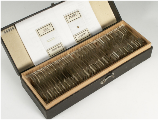
Fig. 4. A complete set of 50 oriented mineral sections prepared by Steeg & Reuter on glass petrographic slides, ca. 1950s.
