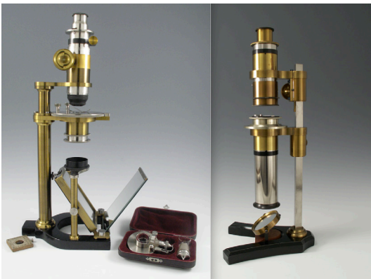
Fig. 5. Early Fuess polariscopes: A conoscope (left) and a stauroscope (right), ca. 1900; both were designed to examine cork-mounted preparations. Conoscopes, with highly converging lenses, were used to examine interference figures. The analyser is a Nicol prism, whereas the polarizer consists of a stack of glass plates and a mirror which provide polarised light via reflection. Stauroscopes (a rare form of orthoscope used to determine precise extinction angles) were utilized to examine mineral sections in orthoscopic light.
