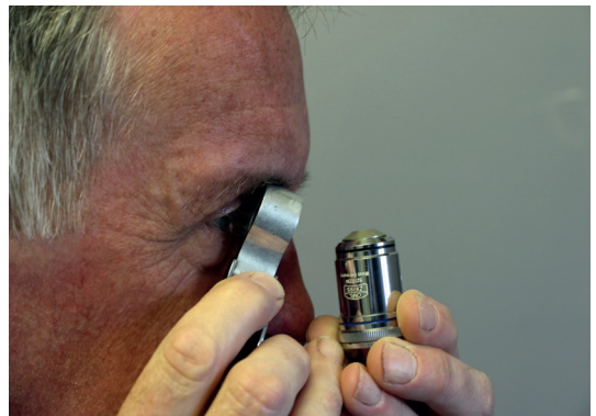
Fig. 2. Inspection of the front lens and tip of an objective using a hand-held loupe of x8 magnification.
