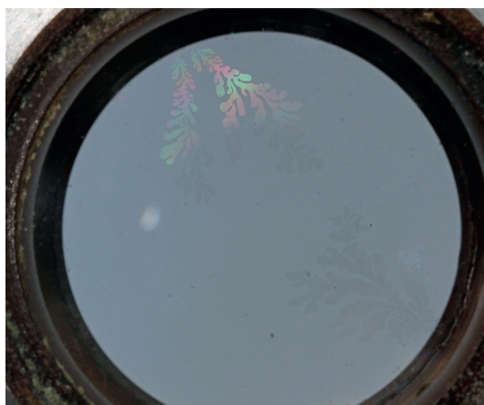
Fig. 5. Dendritic or 'flower' pattern delamination in the front element of a Baker x2.5 objective.
