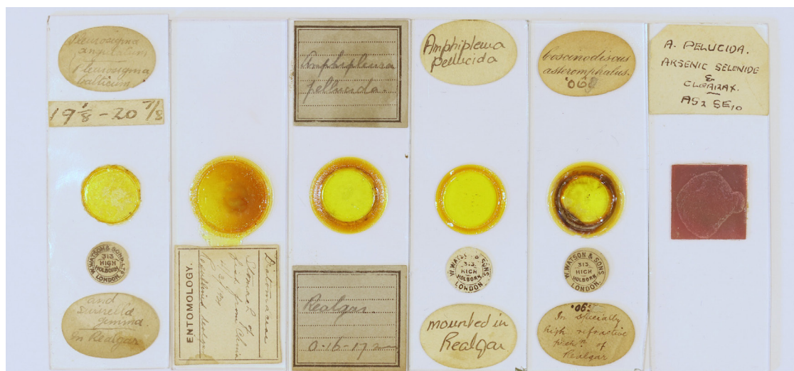
Figure 1c. Slides, from left to right: (13) Watson and Sons Ltd. Pleurosigma angulatum , Pleurosigma balticum , and Surirella gemma . In Realgar. (14) H.C. Wheeler, Montreal, Canada (no makers name on the slide). Diatomaceæ, stomach of fish from China. Dated 4/3/1921(?). In resublimed Realgar. (15) Amphipleura pellucida . Coverslip 0.16-0.17mm. In Realgar. (16) Watson and Sons Ltd. Amphipleura pellucida . In Realgar. (17) Watson and Sons Ltd. Coscinodiscus asteromphalus arrangement. In a specially high refractive preparation of Realgar. (18) Amphipleura pellucida . In Arsenic Selenide, As_2Se_{10} , and Clearax.
