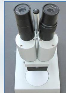
A stereo microscope (left) gives a stereoscopic image; that means we see depth in an image and this is useful for examining a rough piece of rock as the sample can be tilted in different orientations to show the surfaces. The illumination can also be directed to show up specific features.
