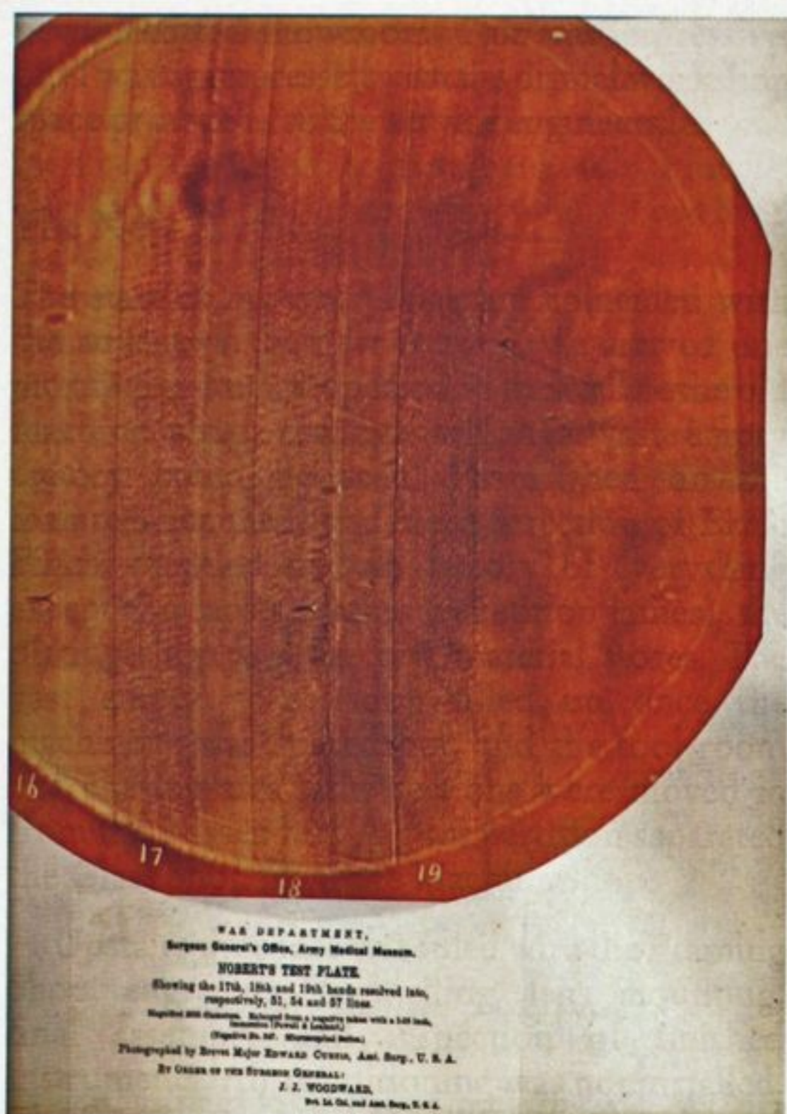
FIG. 21. Woodward photomicrograph of Nobert's test bands numbers 16 to 19.
