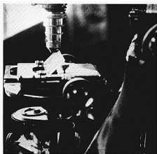
FIG. 4. POWELL & LEALAND MICROSCOPE WITH A 3 \times 1 -IN. SLIDE FOR MEASURING NUMERICAL APERTURE
