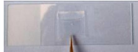
The microscope will usually have objective lenses giving magnifications of ×10 to ×40. With standard ×10 eyepieces the total magnification range is ×100 to ×400. It is now critical that the specimen is as flat as possible and does not move around too much.
